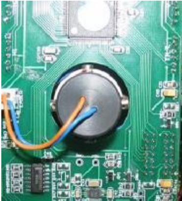
Open the plastic cover of the vertical plate side to reveal built-in laser plummet, as shown, there are four four-hole adjustment screws can be use to adjust the laser plummet, Adjustment procedure is the same as optical plummet.
