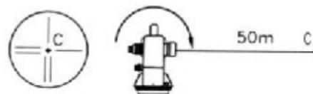
e. Loosen the horizontal motion clamp and tangent screw and revolve the instrument  $180^\circ$  or  $200\text{gon}$ . Fix a sight on point A once more and tighten the motion clamp and screw.
